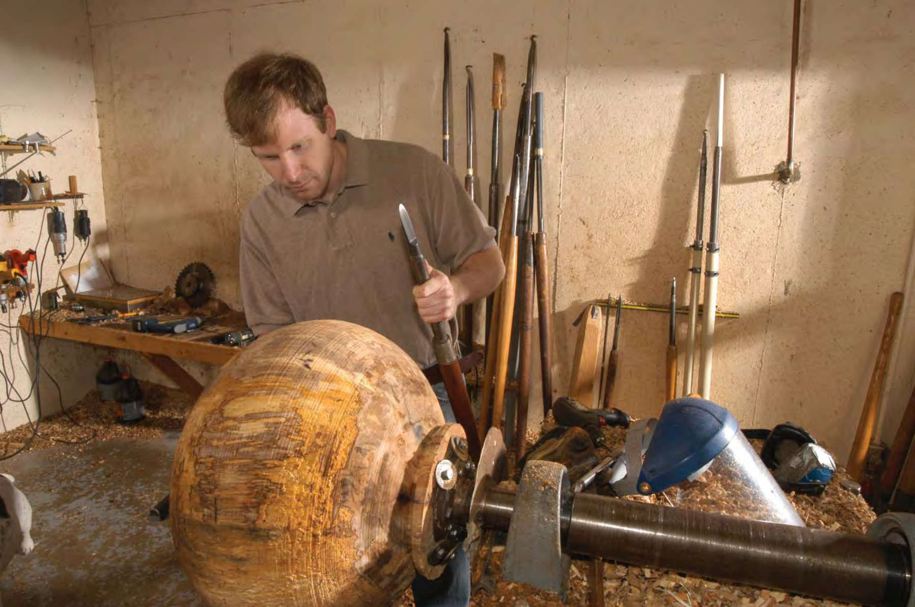
Matt Moulthrop standing at the lathe, holding a lance tool.
